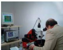
The "on wafer" microwave measurement equipment till 65 GHz purchased by IMT-Bucharest in 2007 in the frame of the National Programme CEEEX (Module 4)
